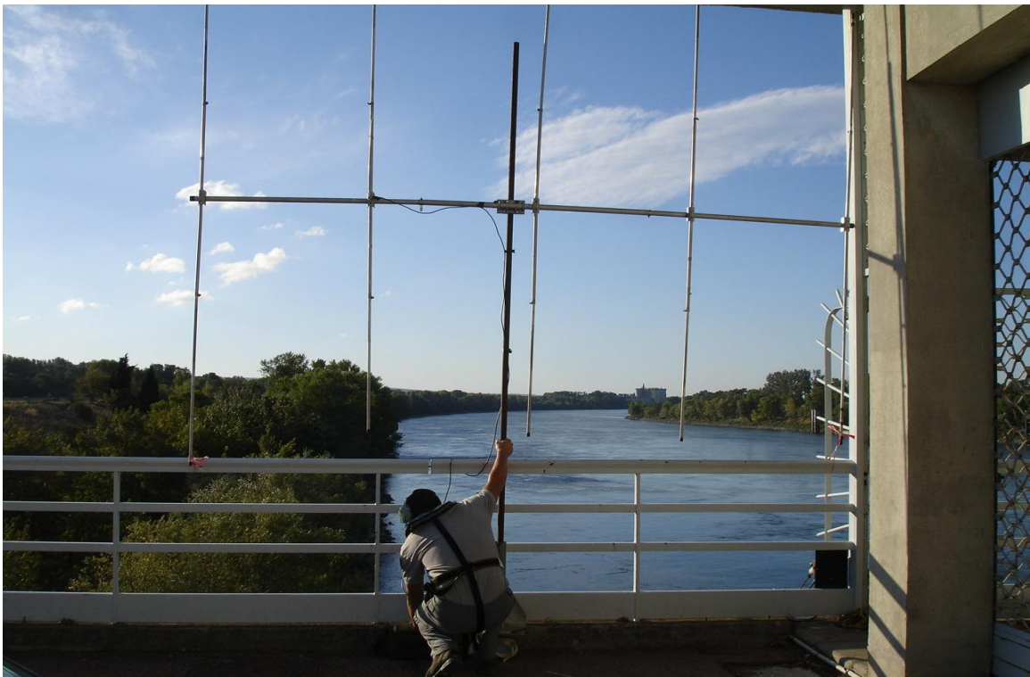
Figure 2-15 Listening for tagged released eels on large Yagi antenna.
