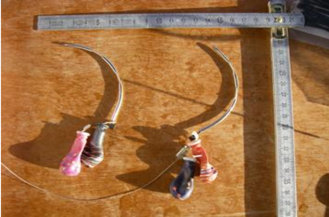
Figure 2-6 Cannula needle with HI-Z balloon tags and ATS radio tag.
